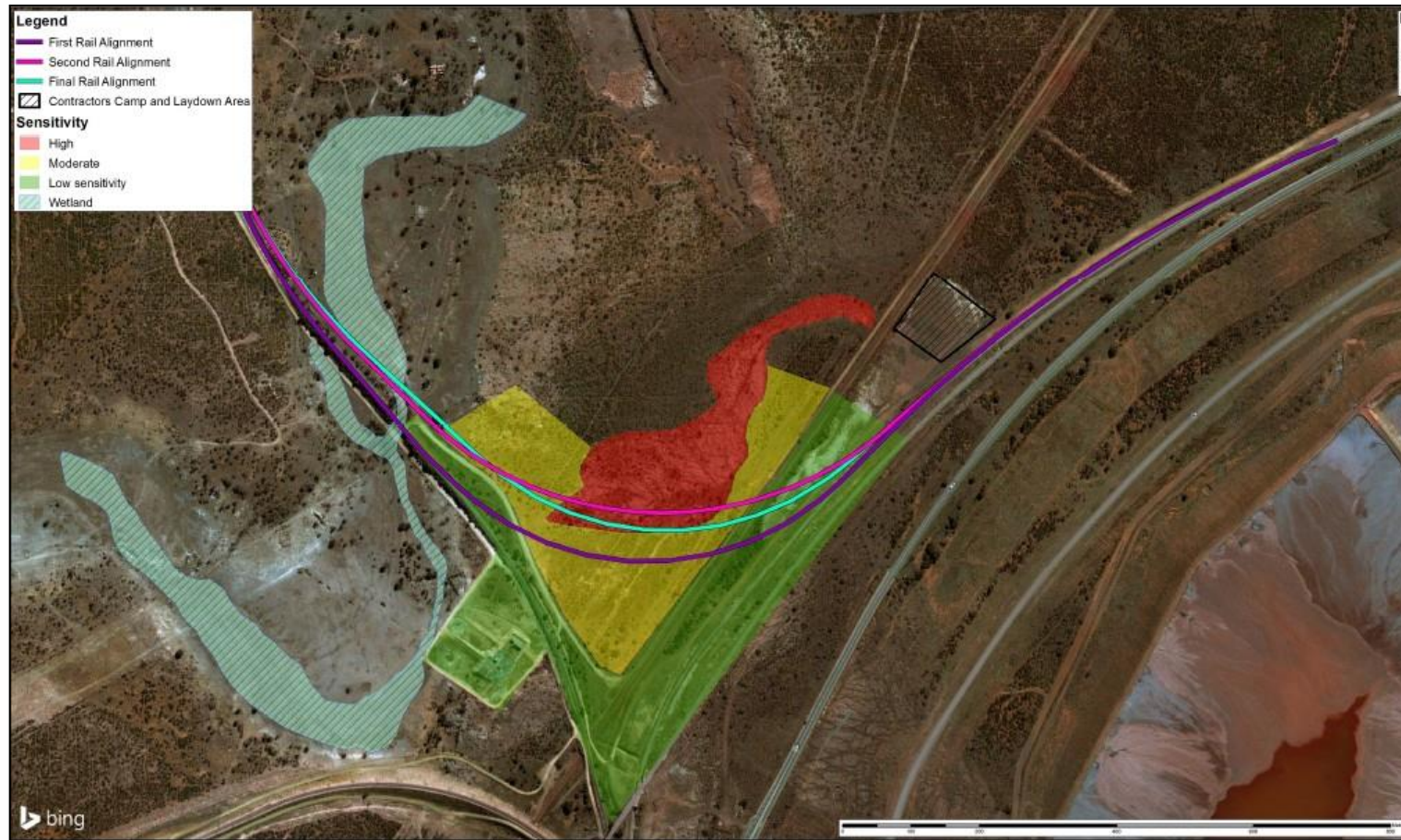
Fig. 2b. Satellite image of the Sishen Transnet Rail Link study area showing route alternatives considered, proposed location of the construction camp and laydown area as well as the current wetland area along the Gamagara River (Image supplied by AECOM).
