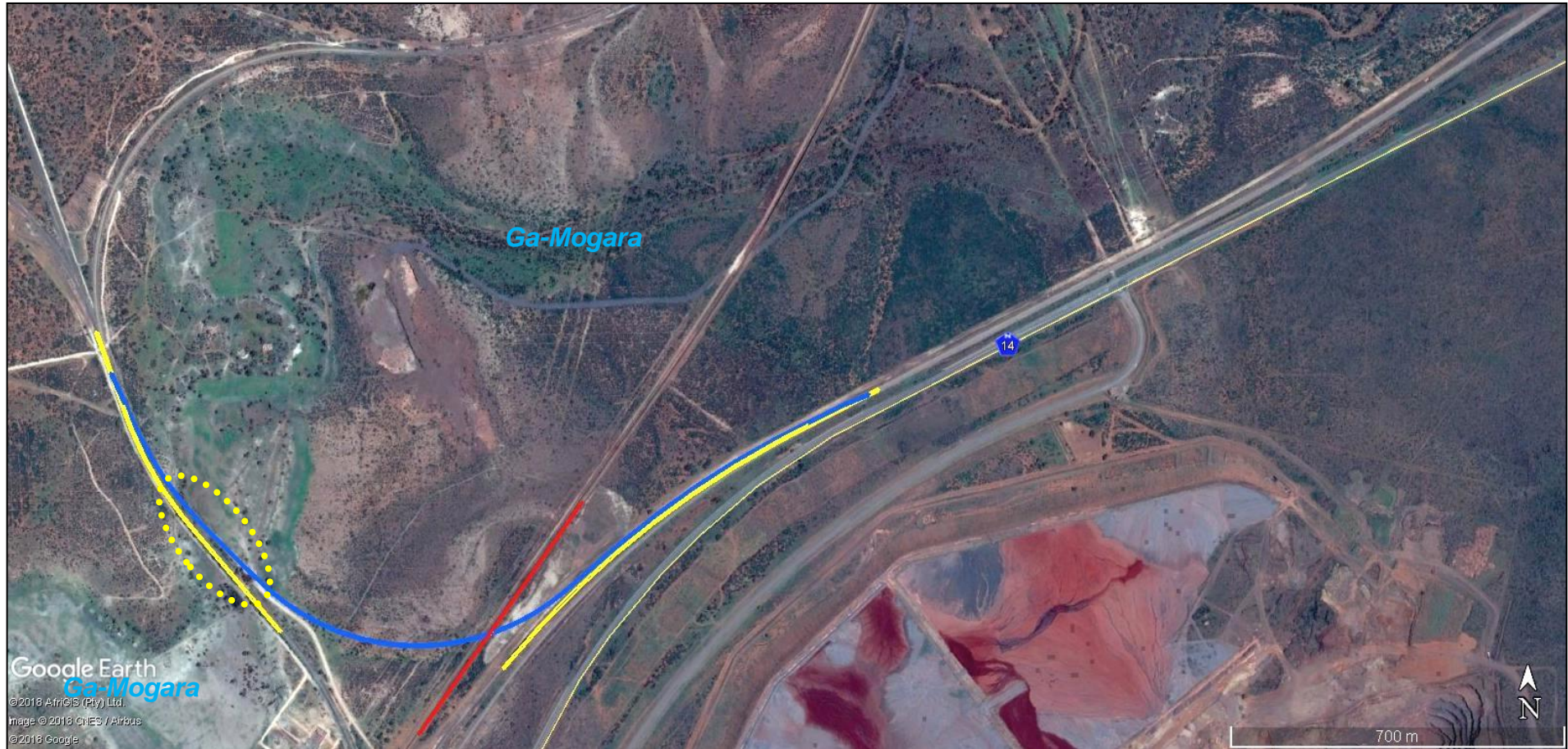
Fig. 2a. Google Earth© satellite image of the study area south of Sishen showing the proposed c. 1 km–long rail link (blue) between two existing railway lines (yellow). Brownish areas are underlain by iron formation while pale cream hues are associated with pedogenic calcrete. The new railway link will traverse the intermittent-flowing Gamagara drainage line (green vegetated zone). The Assmang Khumani open-cast iron ore mine (rusty brown area) is seen to the southeast. The most palaeontologically-sensitive sector of the new rail link is indicated by the yellow dotted ellipse; calcretised alluvium here might be associated with Quaternary mammalian fossils as well as trace fossils and Stone Age artefacts, as seen at Kathu Pan. Note that no substantial excavations into these alluvial deposits are planned.
