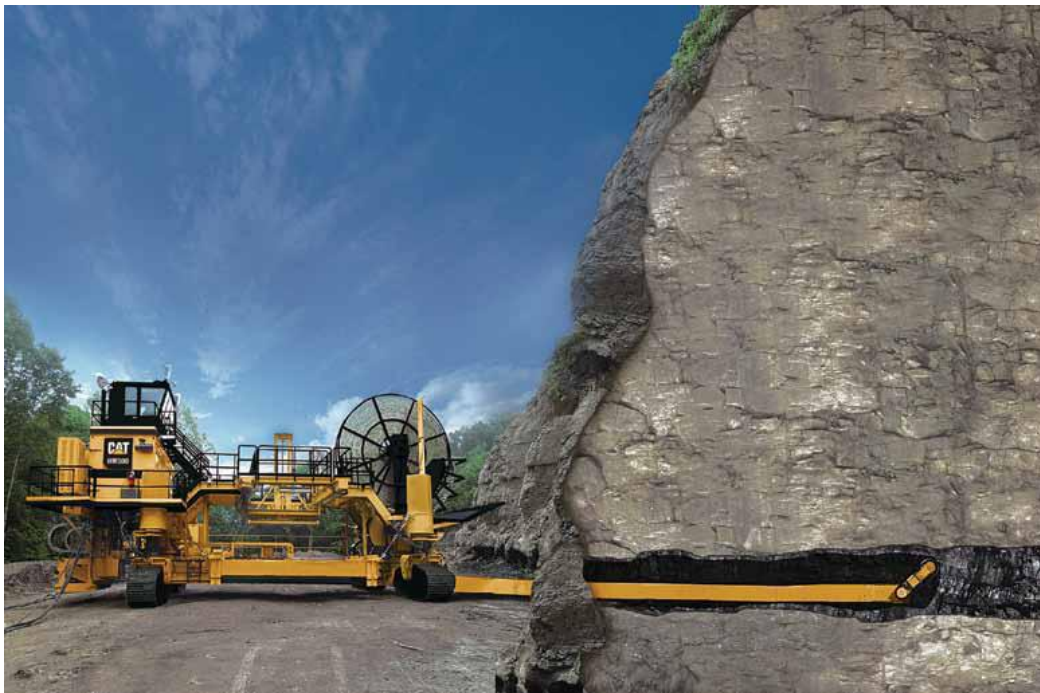
Figure 4a: High wall method of mining (source CAT Brochure). The mining machine extends access the coal seam from an excavated highwall and extends underground for a distance up to 320m. Only the coal is extracted and the overlying strata are not disturbed.
