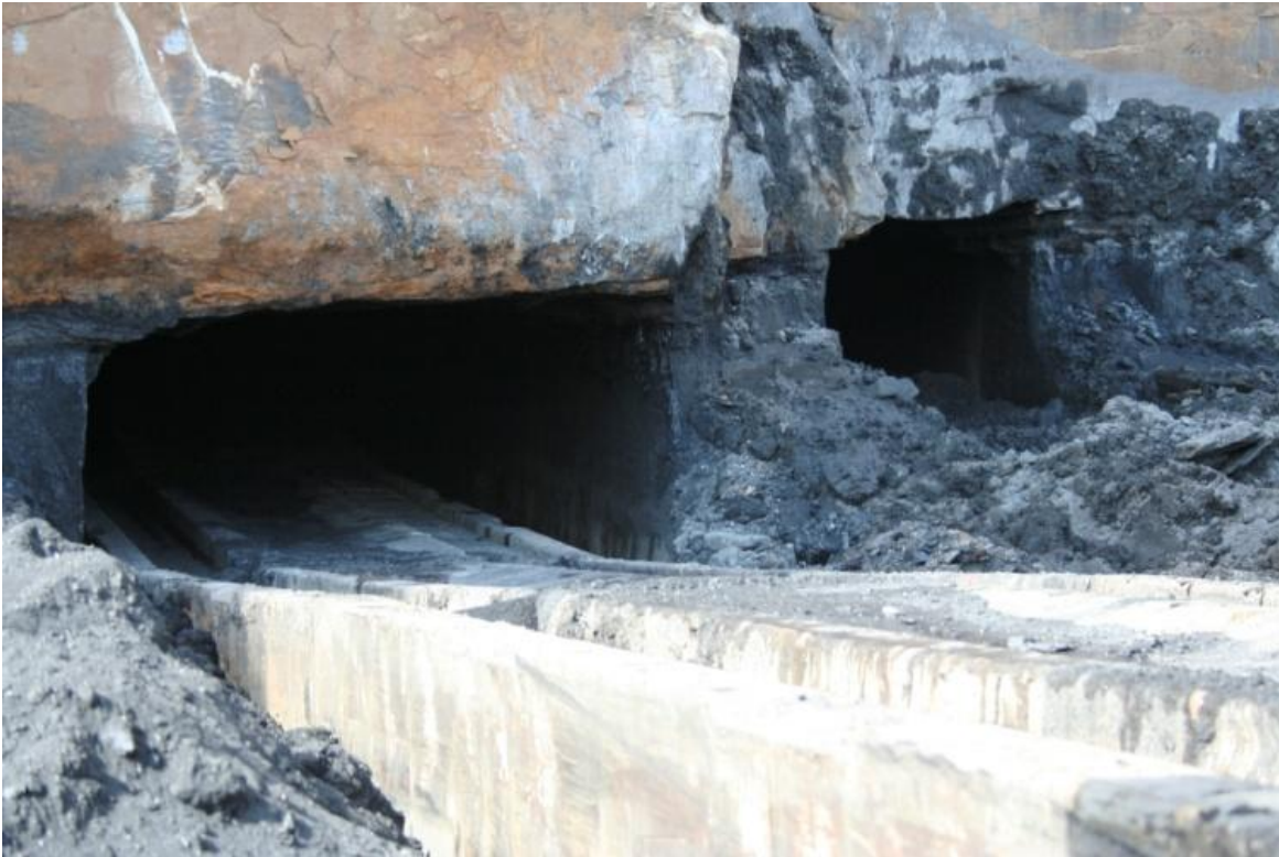
Figure 4b: Photograph taken at the Pocahontas Mine, Kentucky, USA, showing how the highwall miner accesses the coal from a highwall. Note the pillars that remain intact between the successive strips where coal is extracted.
