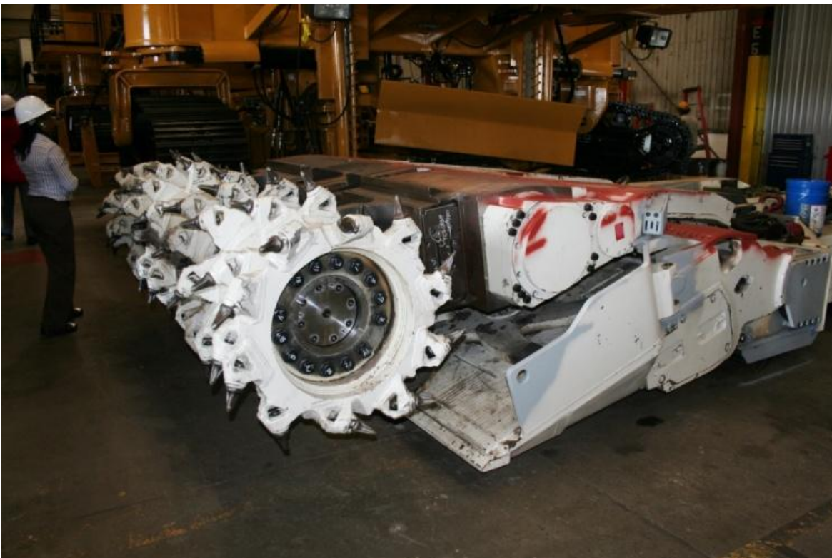
Figure 4c: The continuous miner head that is used to cut the coal for the Highwall miner.
