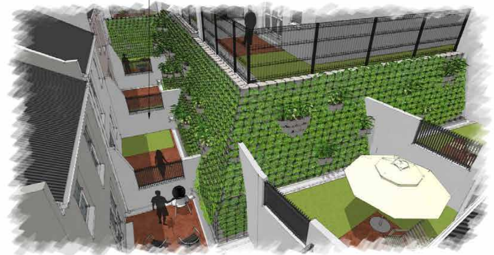
PERSPECTIVE TERRAFORCE WALL - 70° SLOPE
