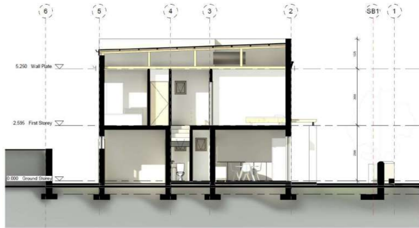
TYPICAL CORNER UNIT - SECTION
