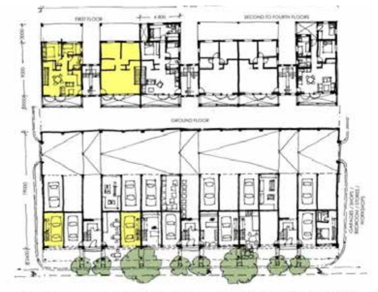
Figure 57. Site development layout sketch showing 4 storey typology with ground floor (below), first floor (top left) and second to fourth floors (top right); yellow shading shows direct access between garage and living space (CNdP, 2022)
