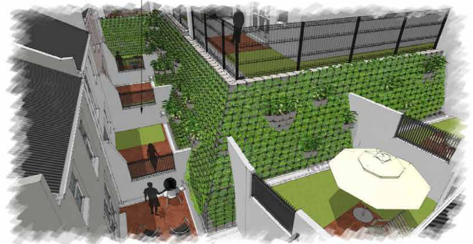
PERSPECTIVE TERRAFORCE WALL - 70° SLOPE
