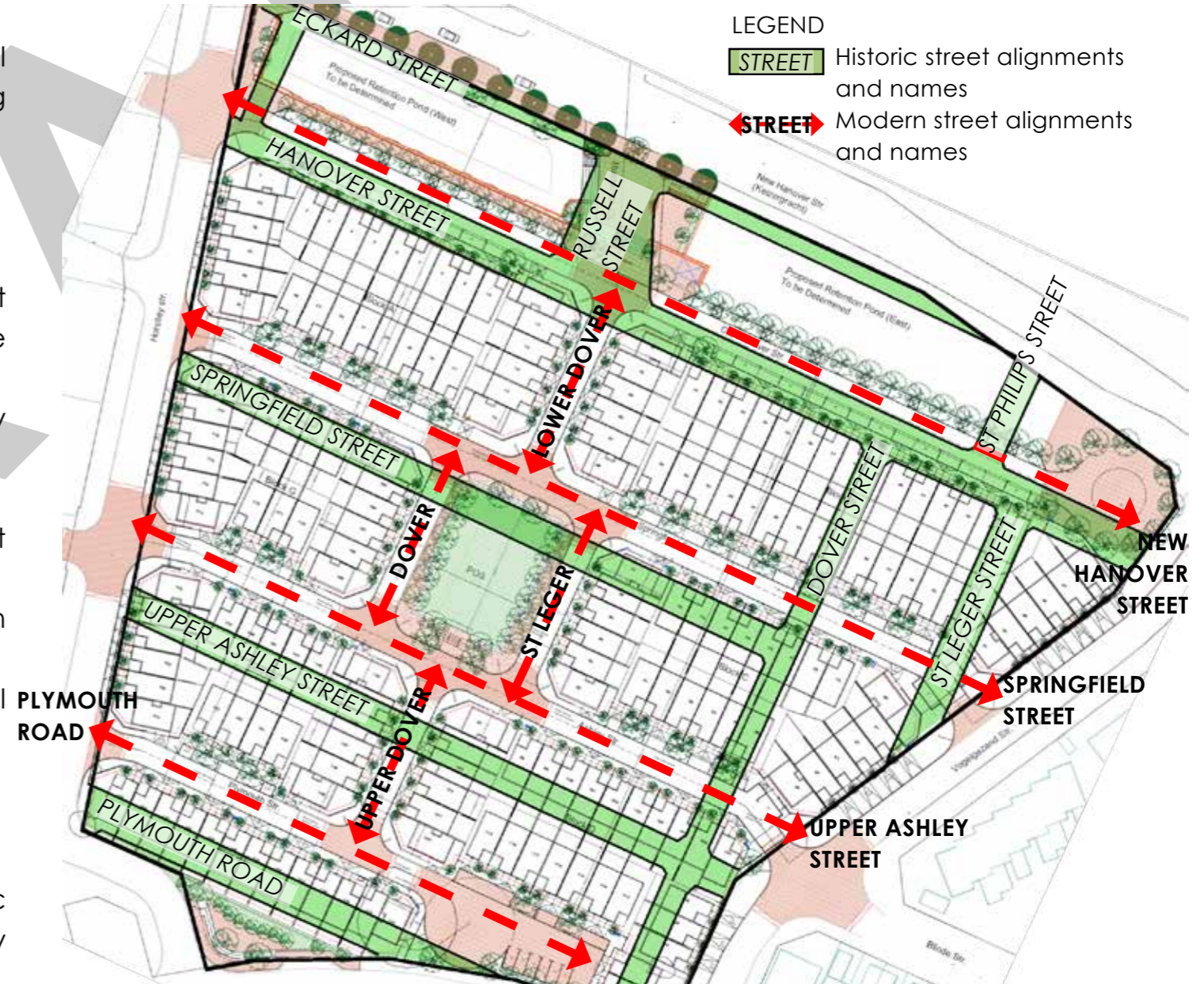
Figure 65. Phase 4 layout showing reinstatement of historic street grid, adapted to accommodate vehicular movement and on-street parking, and reuse of historic street names (RSA, 2022)
