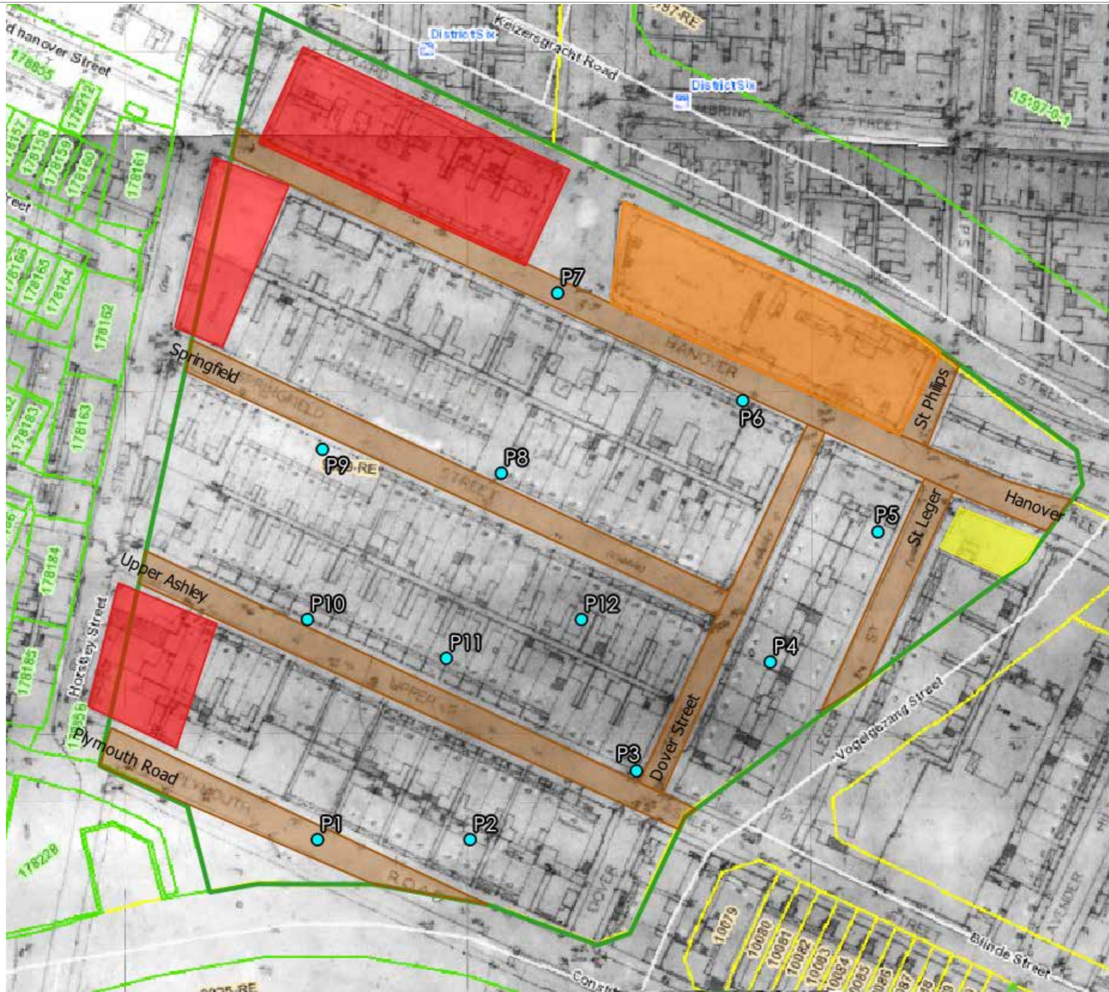
Figure 10. Location of geotechnical test holes and sensitivity mapping overlaid on 1957 City Survey Map for Phase 4 (RSA, 2022)
