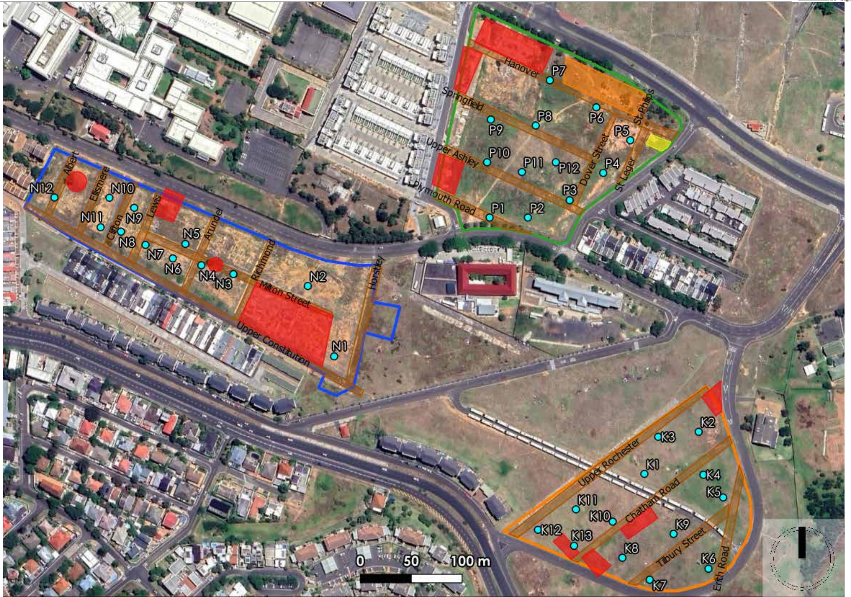
Figure 9. Overlay of geotechnical test holes on the sensitivity mapping for all three parcels (RSA, 2022)
