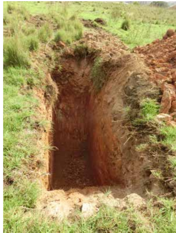
K4 K4 contained disturbed demolition rubble to a depth of 0.9m overlaying a layer of recent rubble to a depth of 1.2m with natural deposits below.
