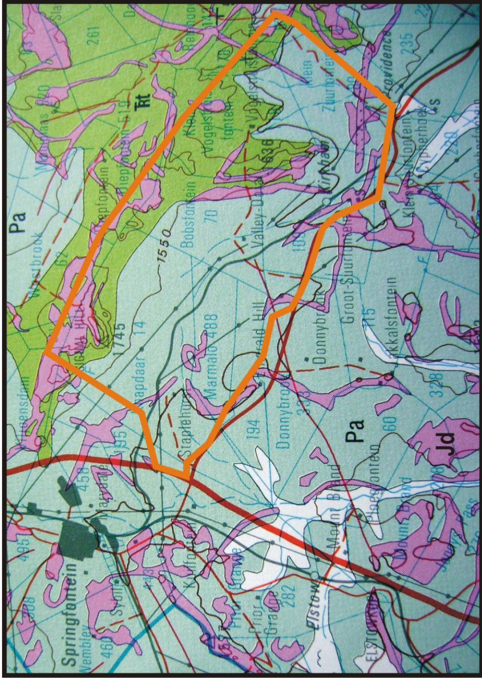
Figure 2. Portion of 1 : 250 000 scale geological map (3025 Colesberg) of the affected area. The geology in the area is represented by late Permian Adelaide ( Pa ) and early Triassic Tarkastad Subgroup sediments ( Trk ), and early Jurassic dolerite intrusions ( Jd ).
