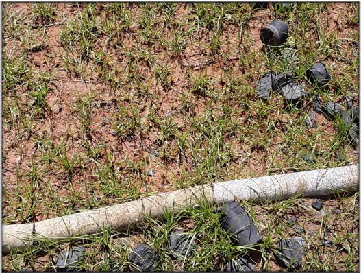
Figure 17: Drill core indicating coal and sediments present in the stratigraphy (-25°55′ 01″ S, 28°57′ 56″ E)
