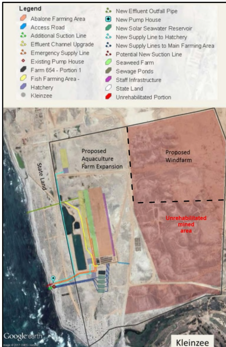
Figure 2. Proposed expansion of the production facilities at Diamond Coast Aquaculture. Adapted from Fig. 2 of Anchor Environmental Consultants, Nov. 2017.
