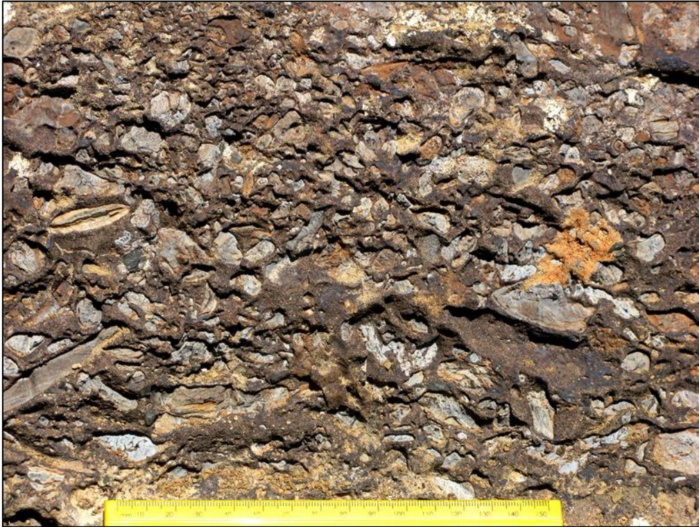
Figure 21. Close-up of the ferruginised breccio-conglomerate seen in the previous figure showing intraclasts of calcrete and calcretised sediment in a brown sandy matrix (Loc 254) (Scale in cm and mm). Such conglomerates might contain transported vertebrate remains.
