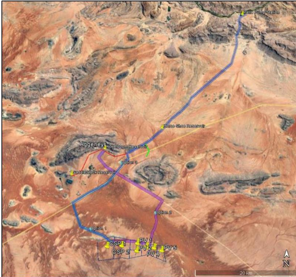
Figure 3: The water pipeline route from the Letsoai CSP 2 to the Orange River. The water pipeline runs alongside the existing water pipeline from the Pelladriфт pump station on the Orange River to the mine at Black Mountain. An alternative option would allow the water pipeline to connect with the Kokerboom Reservoir at Aggeneys.
