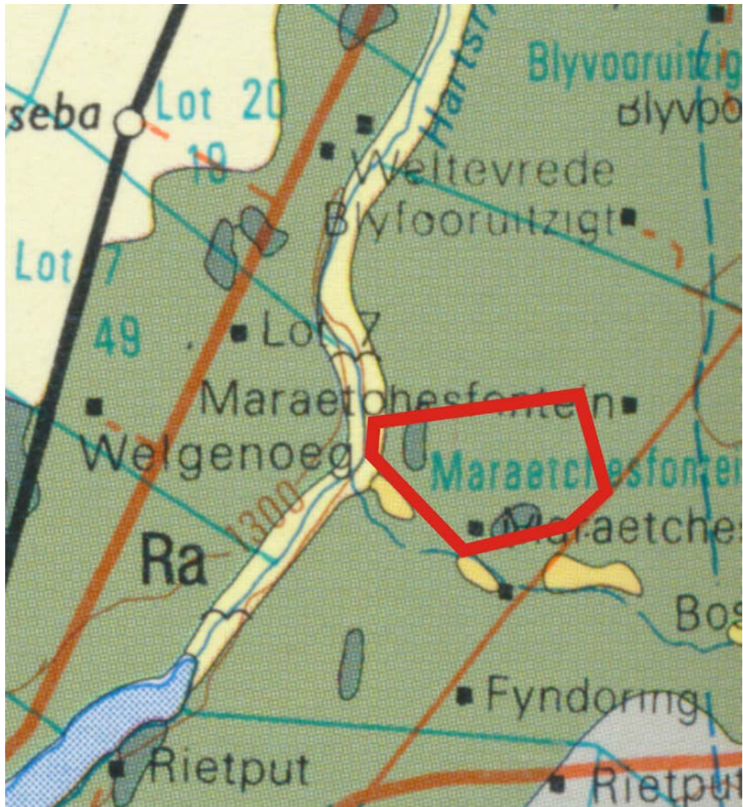
Figure 3. According to the 1:250 000 scale geological map 2724 Christiana, the study area is underlain by Precambrian, Ventersdorp Supergroup lavas of the Allanridge Formation, ( Ra ), that are capped by geologically recent (Quaternary) aeolian sand, alluvium and residual soils.
