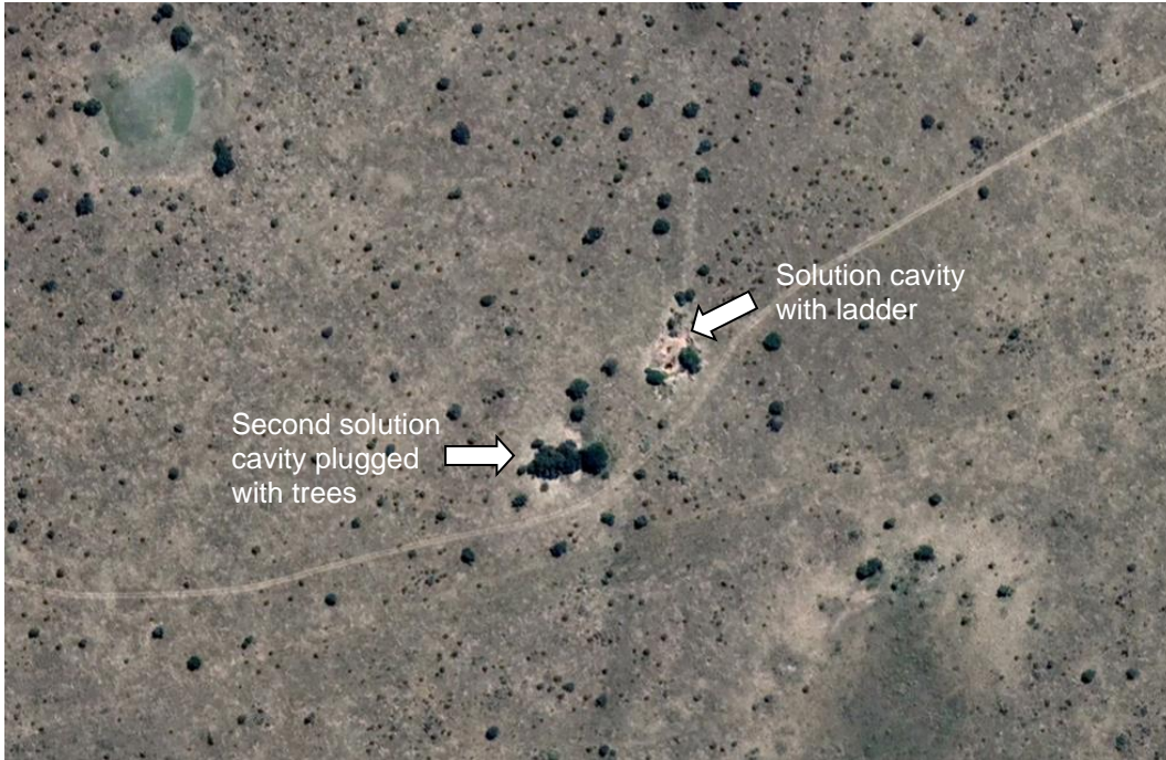
Figure 10e. Two solution cavities/sinkhole – about 50 m apart
