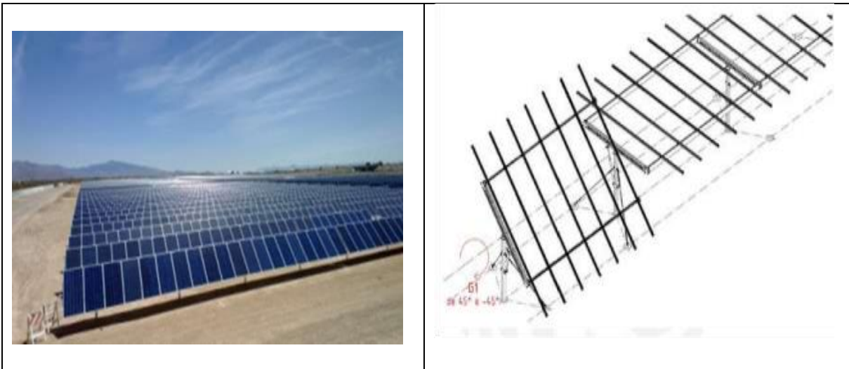
Figure 8: Frame, structural details of a tracking PV technology
