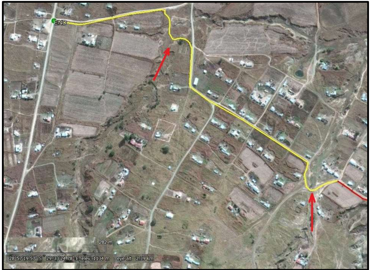
Figure 2: Zoomed in satellite image of the proposed Dabe extension (marked in yellow), and the existing District Road 1239 marked in red. The red arrows show the direction of the water flow and where the two proposed causeways will be built. These zones will likely harbour Stone Age lithics and Quaternary fauna, necessitating the need for a ground survey. Viewed from an elevation of about 2.4 kilometres, North is at the top of the page (Modified Google Earth image, AfriGIS, 2018).
