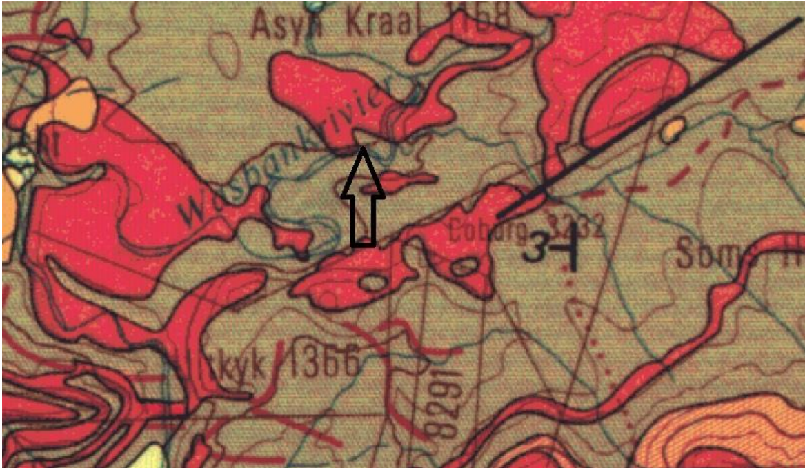
Figure 3: Approximate area of the Dalinkosi Bridge (arrowed). Extract from the 125 000 Geological Map: Dundee 2830. According to this map, the bridge crosses Vryheid Formation (Pv: grey).
