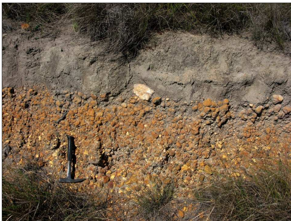
Fig. 21. Well-sorted conglomerate of rounded, ferruginised sandstone pebbles and ferricrete nodules overlain by grey silty soil with sparse, angular vein quartz clasts, R62 road cutting (Loc. 049).
