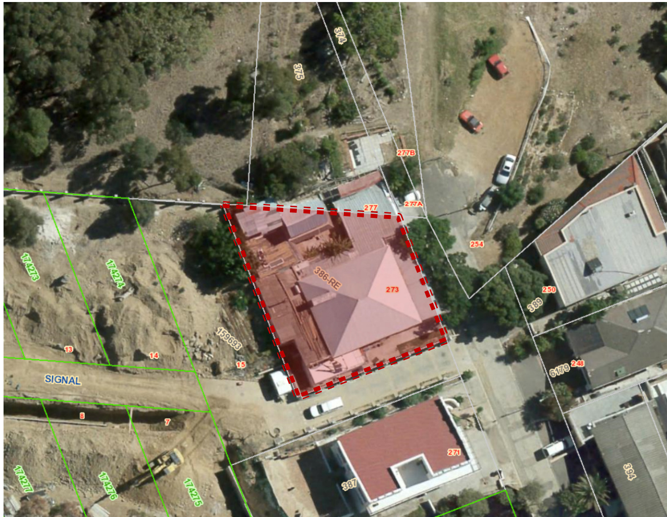
Figure 4: Image illustrating the location and extents of erf 386-RE on Longmarket Street. Note some building structures located on the north erf boundary of erf 386-RE encroach on erf 375. (Source: [Online]. Available: http://maps.capetown.gov.za/isisiv/ [22 July 2016].)
