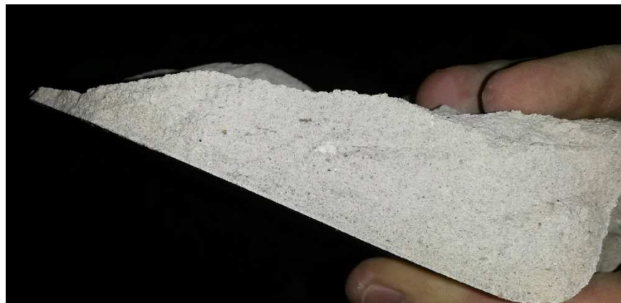
Photo 4.5.8 40mm thick cementitious plaster
