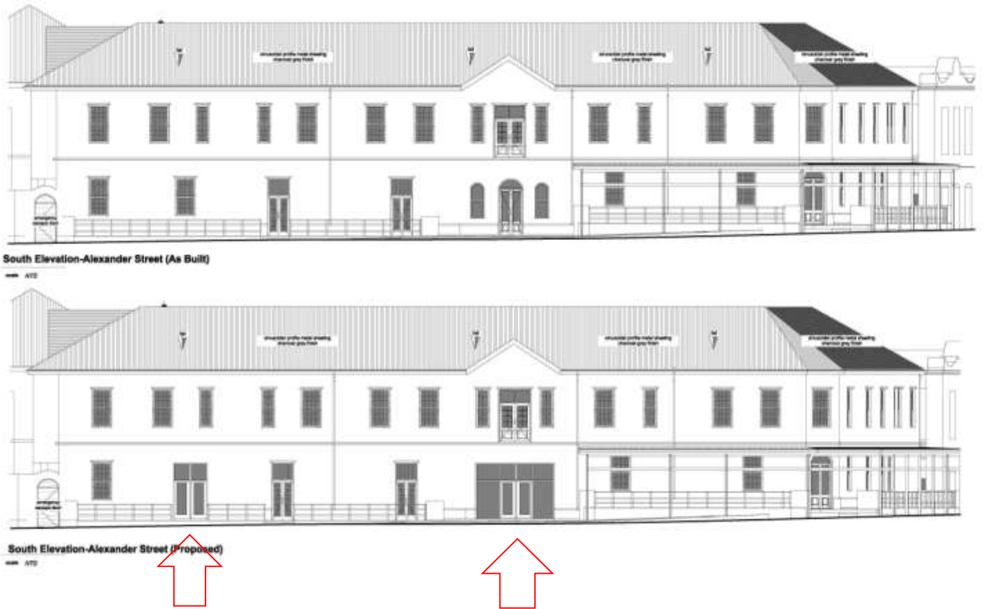
Figure 12: Proposed Alexander Street elevation: existing (above) and proposed (below) (DHK Architects)
