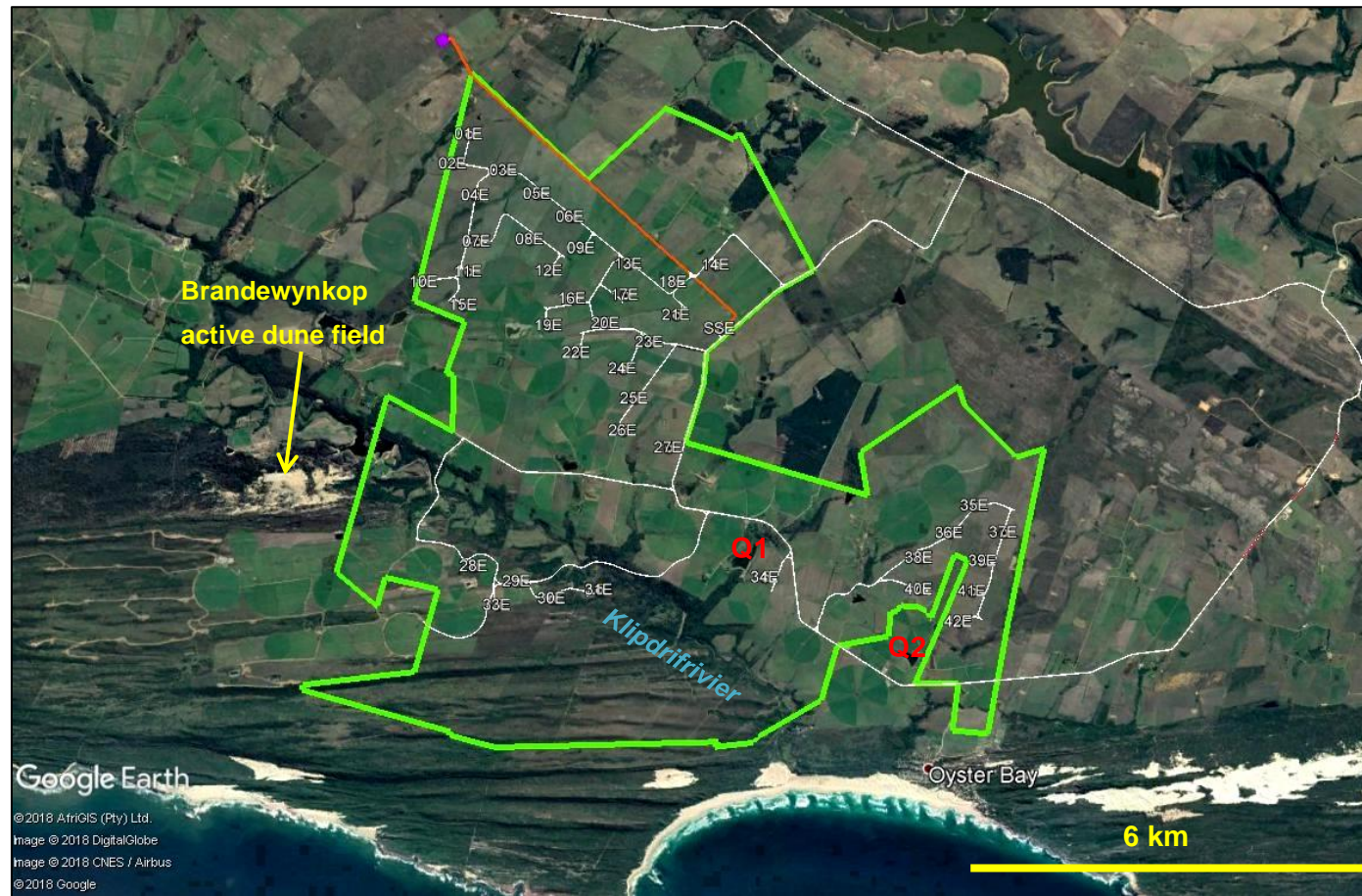
Figure 3. Google Earth© satellite image of the Impofu East Wind Farm study area (green polygon) spanning the coastal platform c. 20 km southwest of Humansdorp. The provisional development footprint is indicated, including wind turbine and standing area positions (numbered), access roads (white) and 132 kV line (orange) from the on-site Impofu East Substation (small blue square) to the collector substation (purple). Q1 and Q2 (red) indicate two sites of geological / palaeontological conservation value, only one of which lies within the wind farm project area (See Fig. 6 for more detail).
