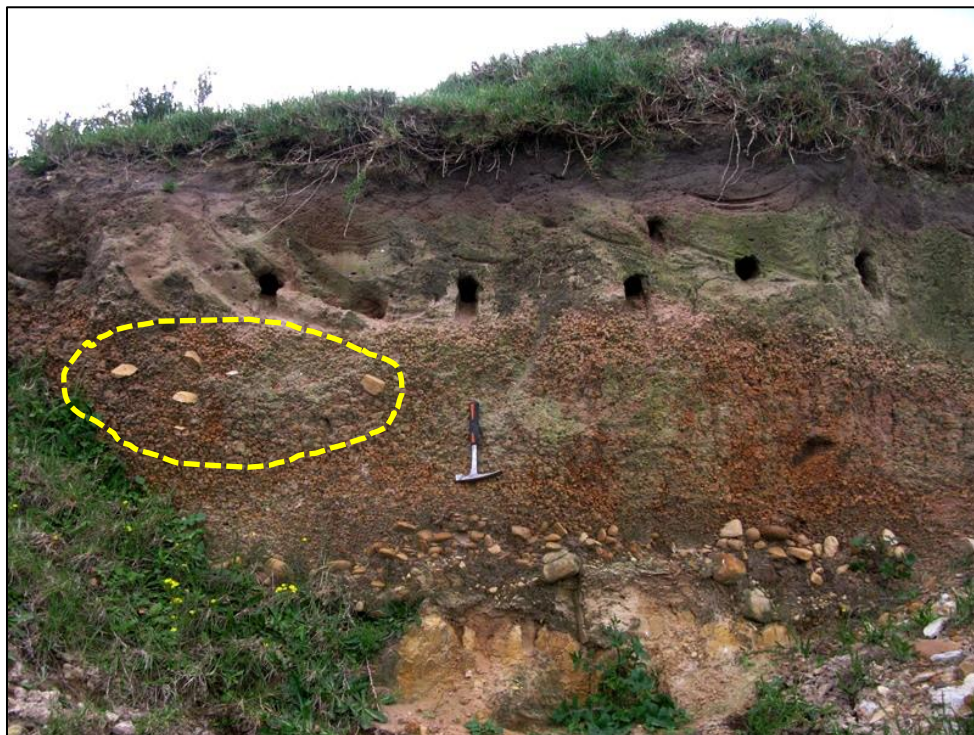
Figure 17. Quarry Q2 on Slange Rivier 733 (just outside the Impofu East Wind Farm study area) showing weathered Cape Supergroup bedrocks overlain by thin pebbly conglomerate and then well-developed nodular ferricrete within the base of the Pleistocene Nanaga Formation John E. Almond (2017) Natura Viva cc
