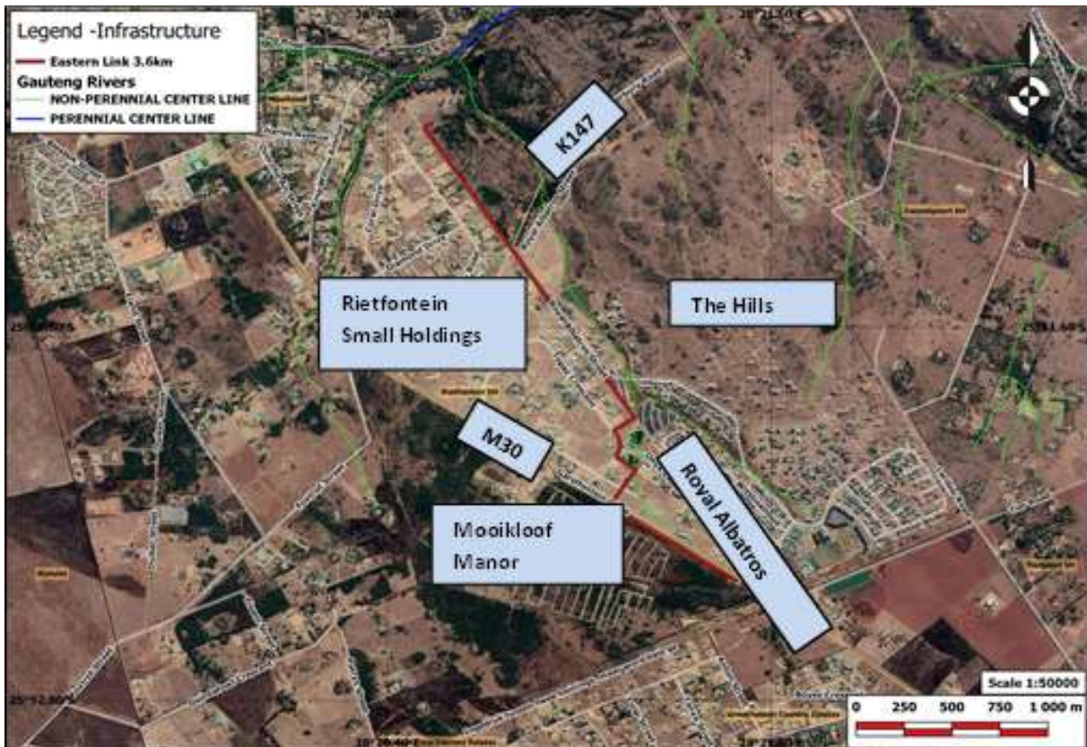
Figure 2: Location Map. Eastern Link Sewer Line indicated in red (courtesy Bokamoso Landscape Architects & Environmental Consultants CC).
