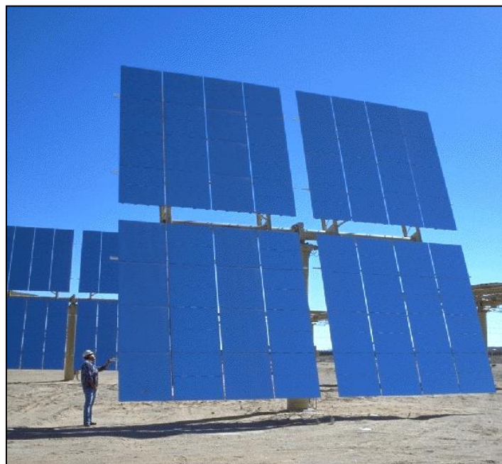
Figure 4 - Single heliostat – image courtesy NREL
