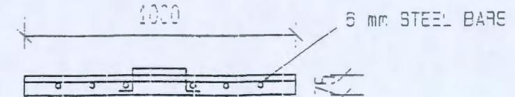
DETAIL OF TYPICAL PIT SEALING BLOCK (scale 1:20)
