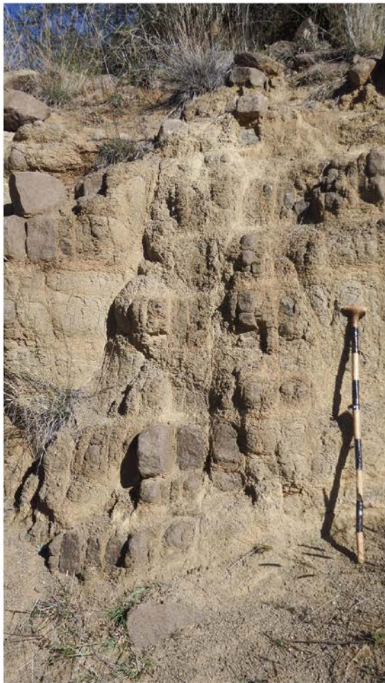
Figure 7. The site is underlain by intrusive Jurassic dolerites (Karoo Dolerite Suite) and associated contact metamorphic metasediments. Scale 1 = 10 cm.
