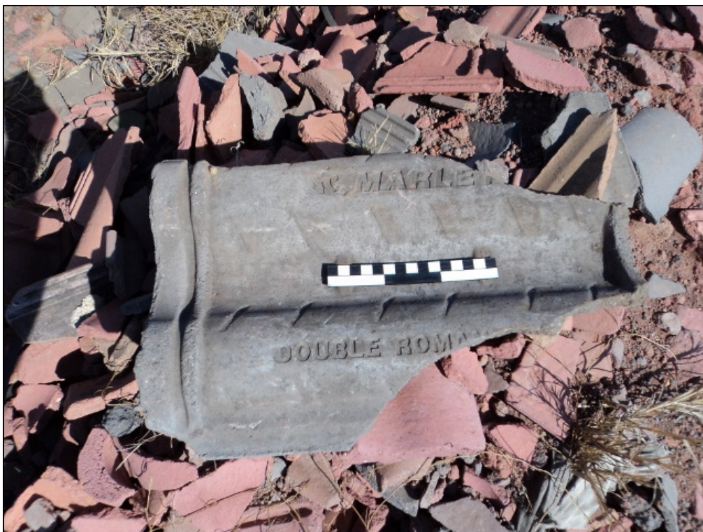
Figure 16: Double Roman roof tiles produced by Marley.
