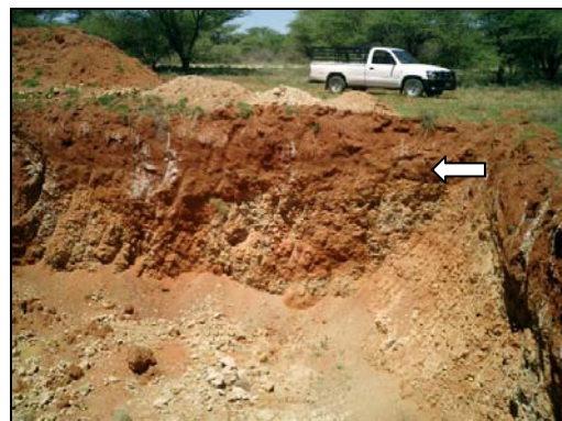
IMAGE 6: Section at quarry pit VH002 indicating the position of the LSA member within the stratigraphy
