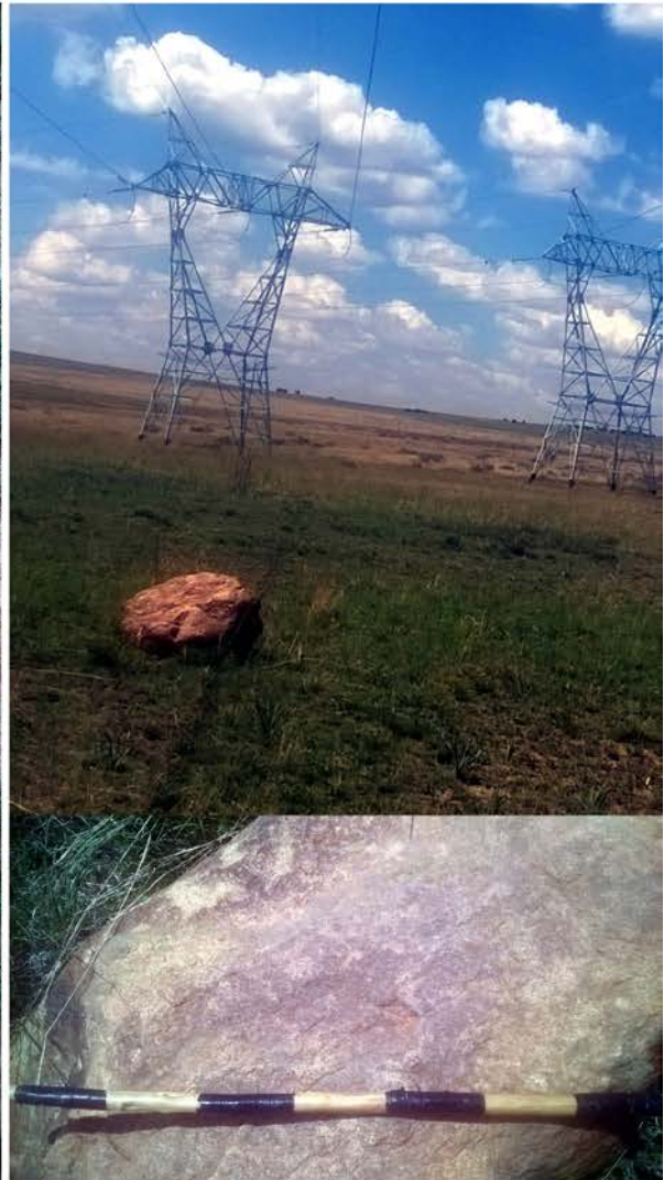
Figure 7. The site is located on flat open grassland capped by a gravelly residual soil (below left) underlain by coarse to medium-grained granite (below right). Scale 1 = 10cm.
