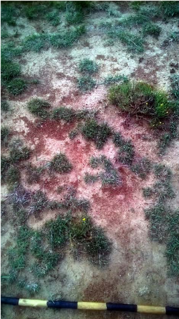
Figure 7. The site is located on flat open grassland capped by a gravelly residual soil (below left) underlain by coarse to medium-grained granite (below right). Scale 1 = 10cm.
