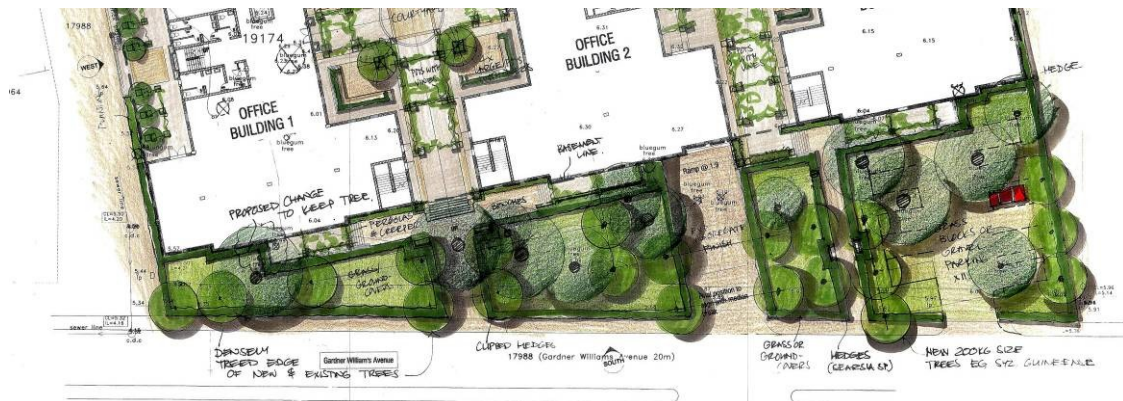
Figure 19: Detail from the Landscape Concept Plan indicating the densely treed southern edge of new and existing trees
