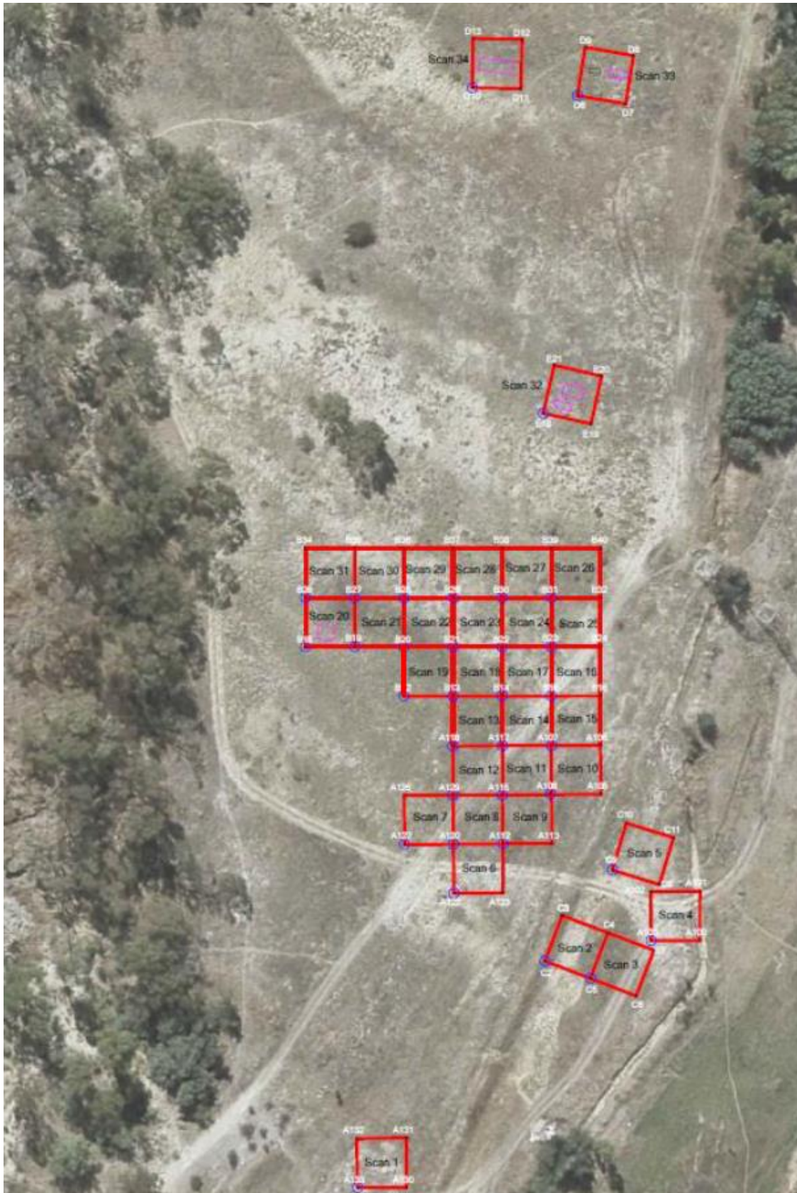
Figure 6-8: Location of GPR Scan Grid
