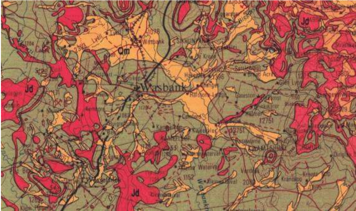
Figure 2: Extract from the Dundee 2830 1: 250 000 scale Geological Map. Red is dolerite, brown is the Vryheid Formation and orange the Masotcheni Formation.
