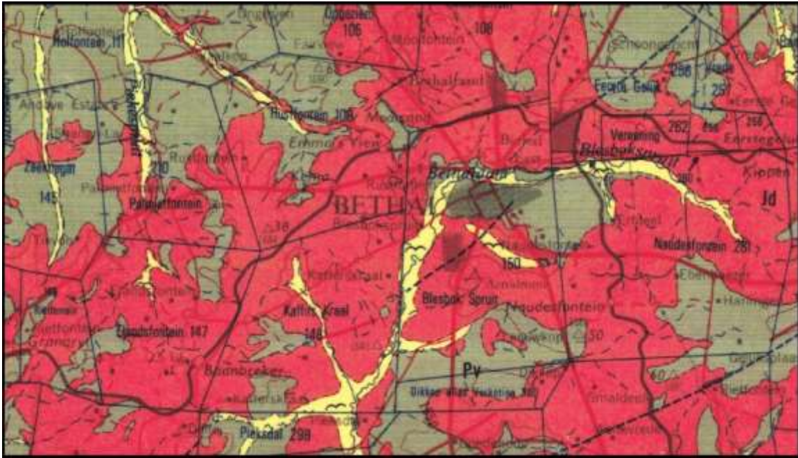
Figure 2: Extract from the East Rand (2628) 1: 250 000 scale Geological Map. Red is dolerite and yellow is alluvium.
