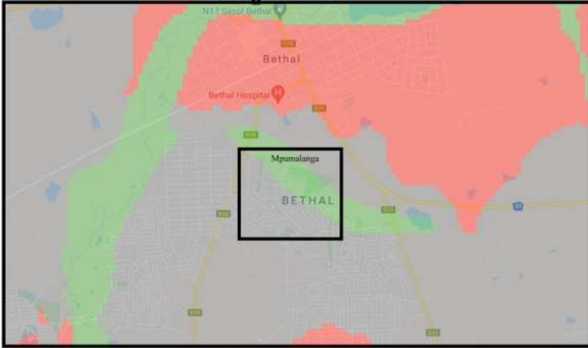
Figure 3: Extract from SAHRIS PalaeoSensitivity Map showing a zoomed-in section of the Emzisoni development area (boxed). The bulk of the area is grey (Dolerite) with alluvium in green. According to the Sahriss Palaeosensitivity map only a Desk-Top PIA is required.
