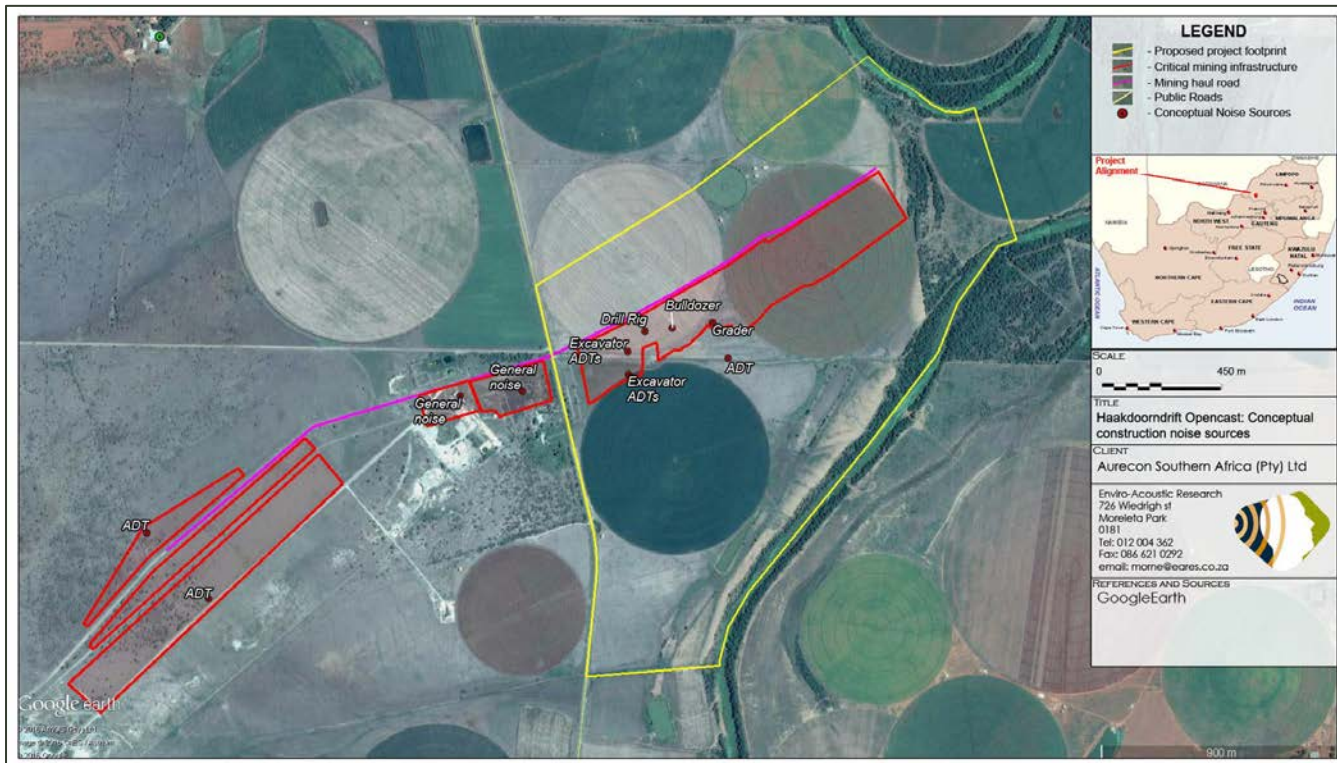
Figure 87 | Potential noise sources during the construction phase (EAR, 2016).
