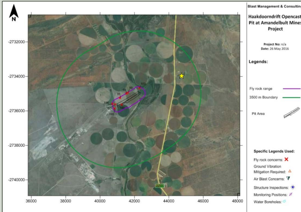
Figure 95 | Fly rock boundary of 268 m around the general pit area, relative to True North Aviation Hub, indicated as a star to the northeast of the pit (Blast Management & Consulting, 2016).
