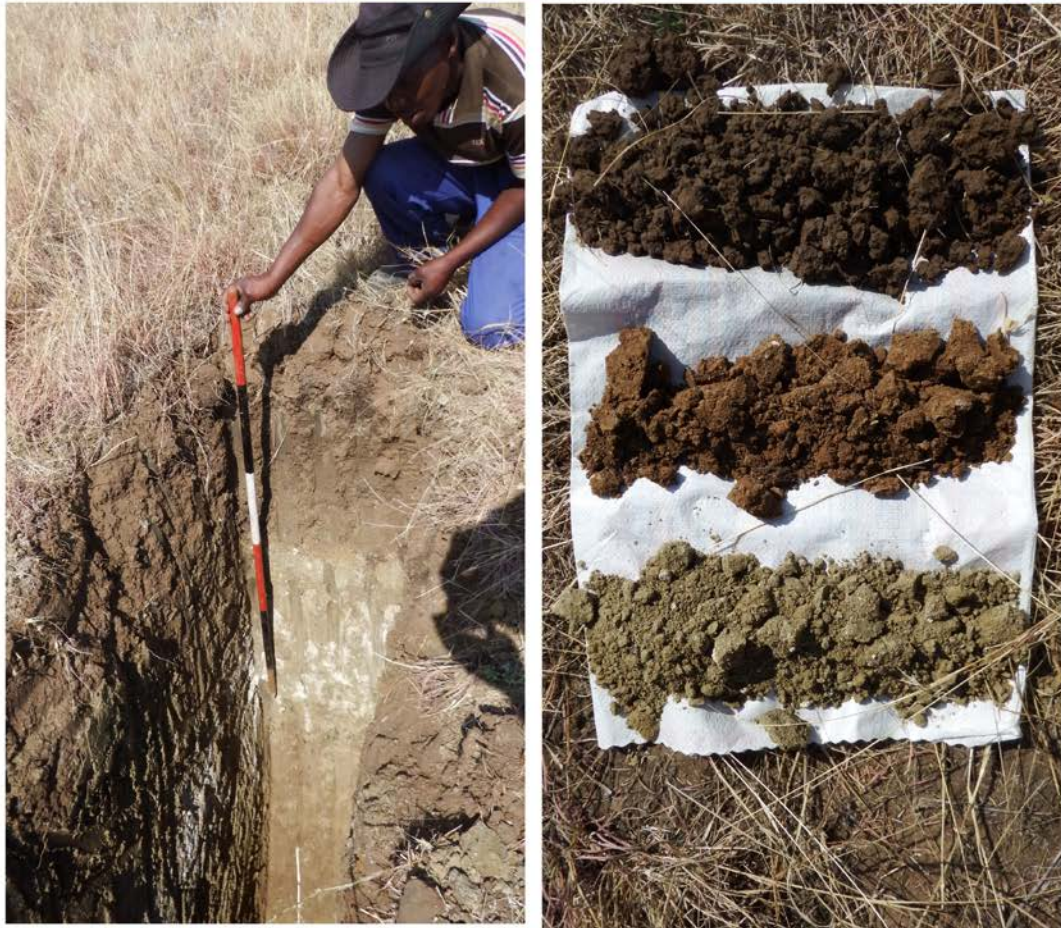
Figure 5. The size of each test pit was about 1 m wide x 4 m long x 2-3 m deep and were filled up immediately after each inspection. Scale 1 = 30 cm.
