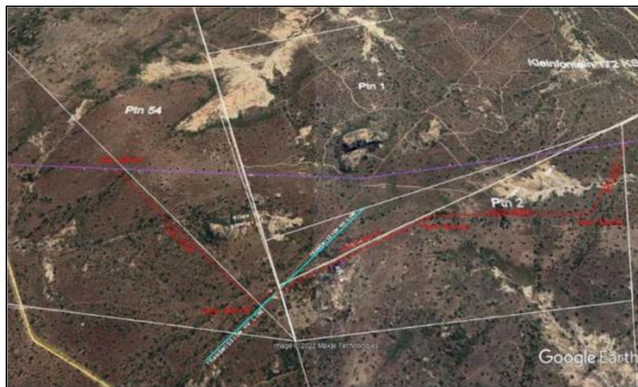
Figure 11 - Bend 3-6 (red line) which is a proposed deviation from the authorised (Source: client).
