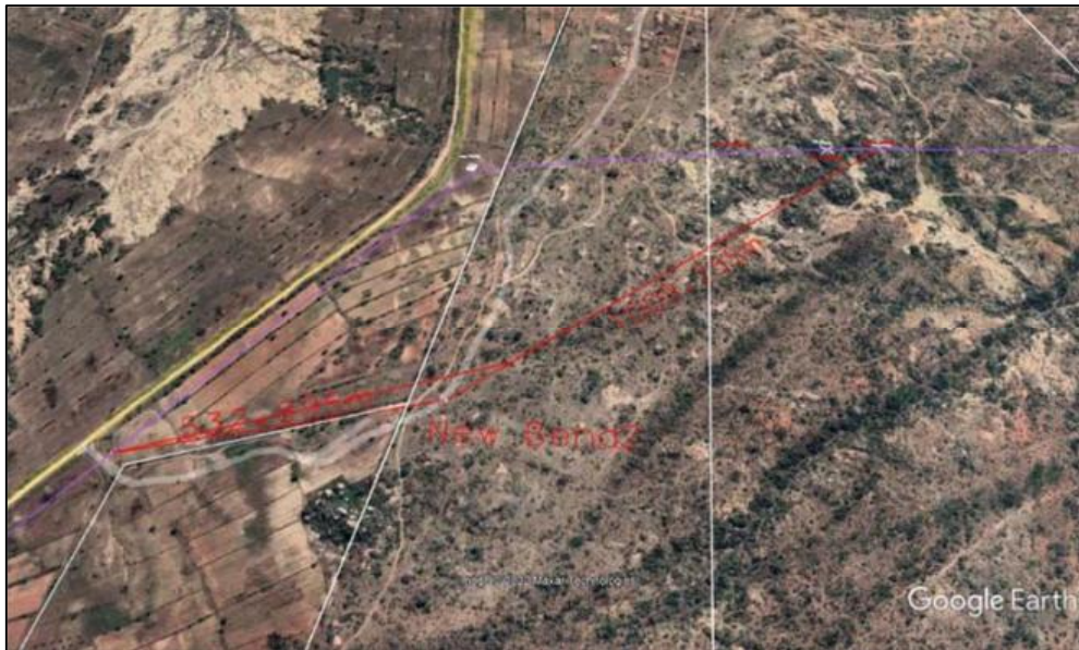
Figure 9 - Bend 2 (red line) which is a proposed deviation from the authorised alignment (purple line) (Source: client).
