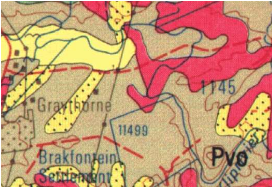
Figure 2 (a): Extract from the Harrismith (2828) 1: 250 000 Geological Map. Grey (Pvo) is the Volksrust Formation, red is Karoo Dolerite and the yellow is Quaternary sediments.
