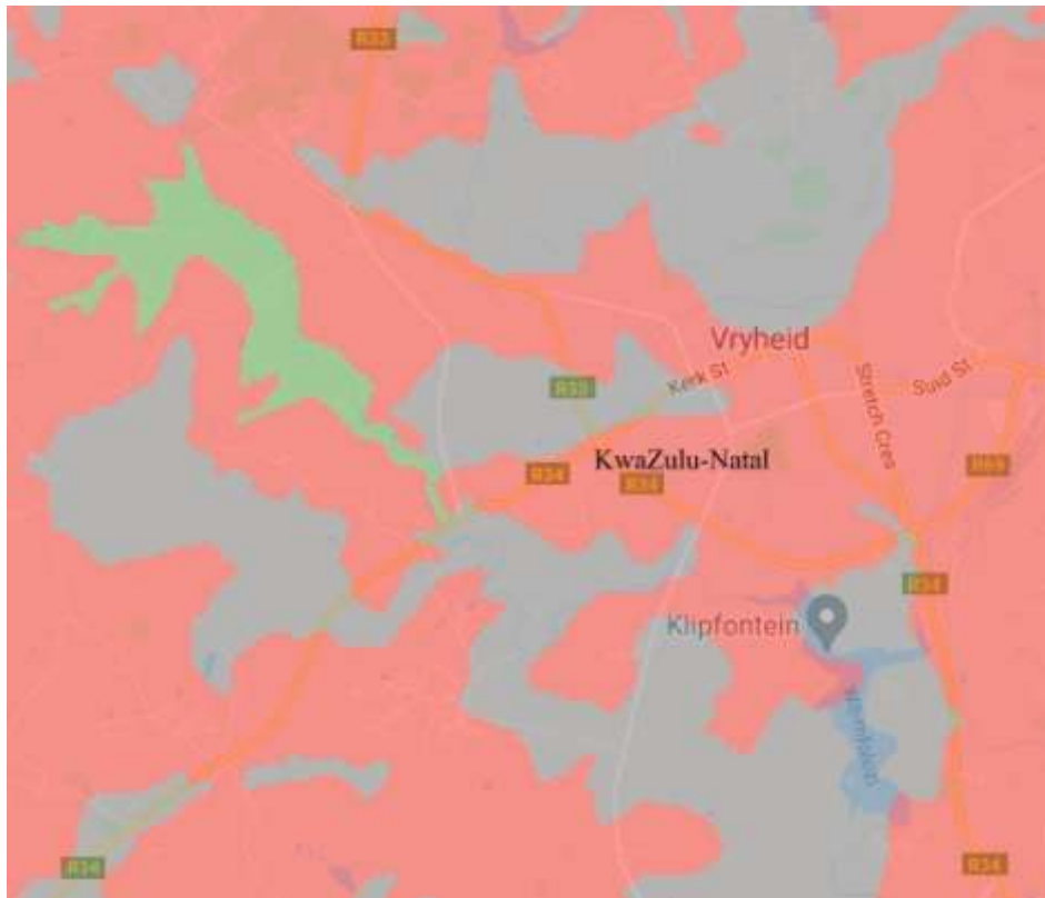
Figure 4: Palaeosensitivity of the Hartbeesbult Sustainable Farm area. Red represents Vryheid Formation, Green represents alluvial deposits and Grey the Karoo Dolerite. See Table 1 for palaeosensitivity codes.
