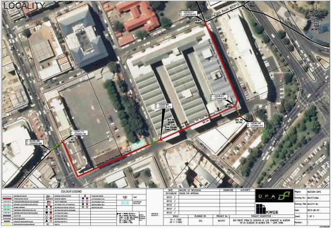
Figure 1: The proposed fibre optic duct route in the CBD Somerset Road - Hospital Street (red line).
