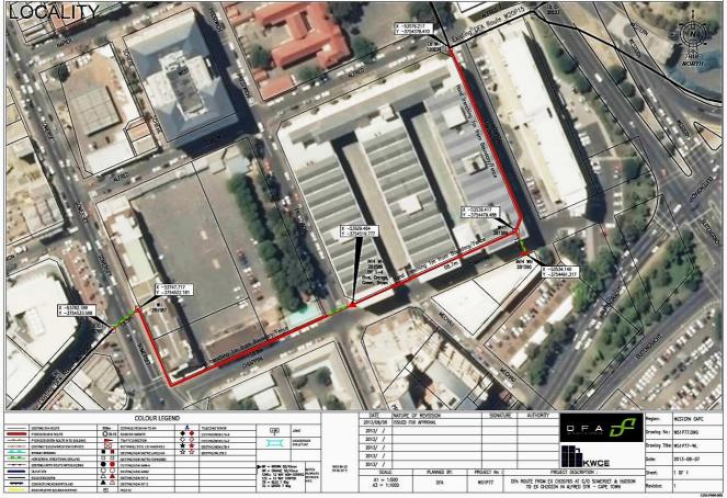
Figure 1: The proposed fibre optic duct route in the CBD Somerset Road - Hospital Street (red line).
