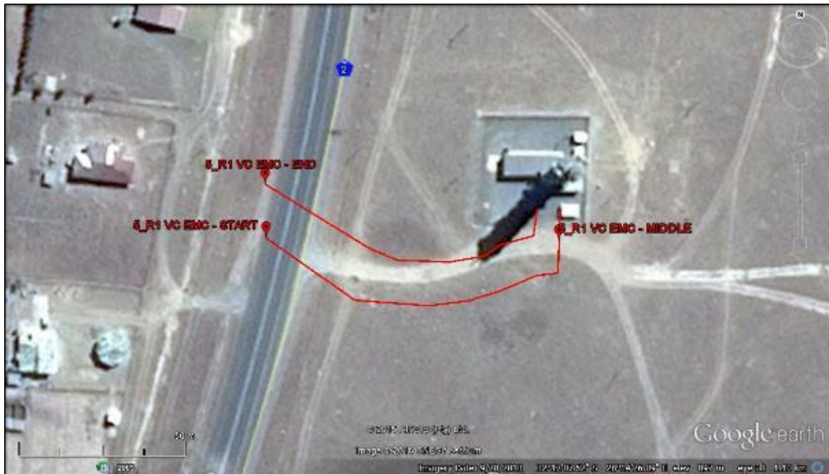
Figure 42. Aerial view of the deviation route for Repeater Site R1 VC EMC, located off the N2 national road.
