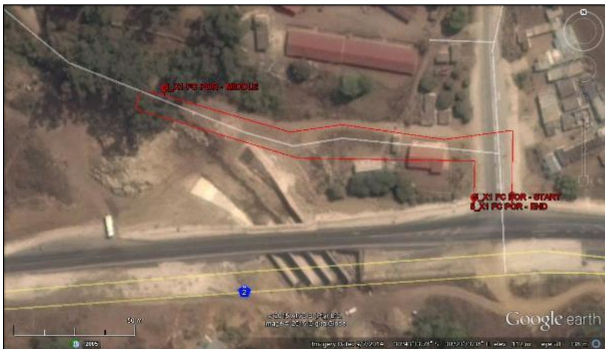
Figure 58. Aerial view of the deviation route for Repeater Site X1 FC POR situated off the N2 national road on the western outskirts of Port Shepstone.
