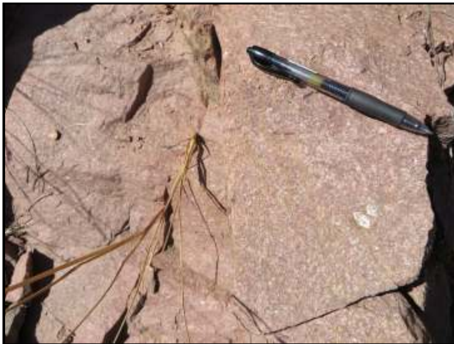
Figure 6: Pink, medium grained igneous rock of the Rooiberg Group cropping out at the historical quarry (Waypoint BM01, see Figure 2).
