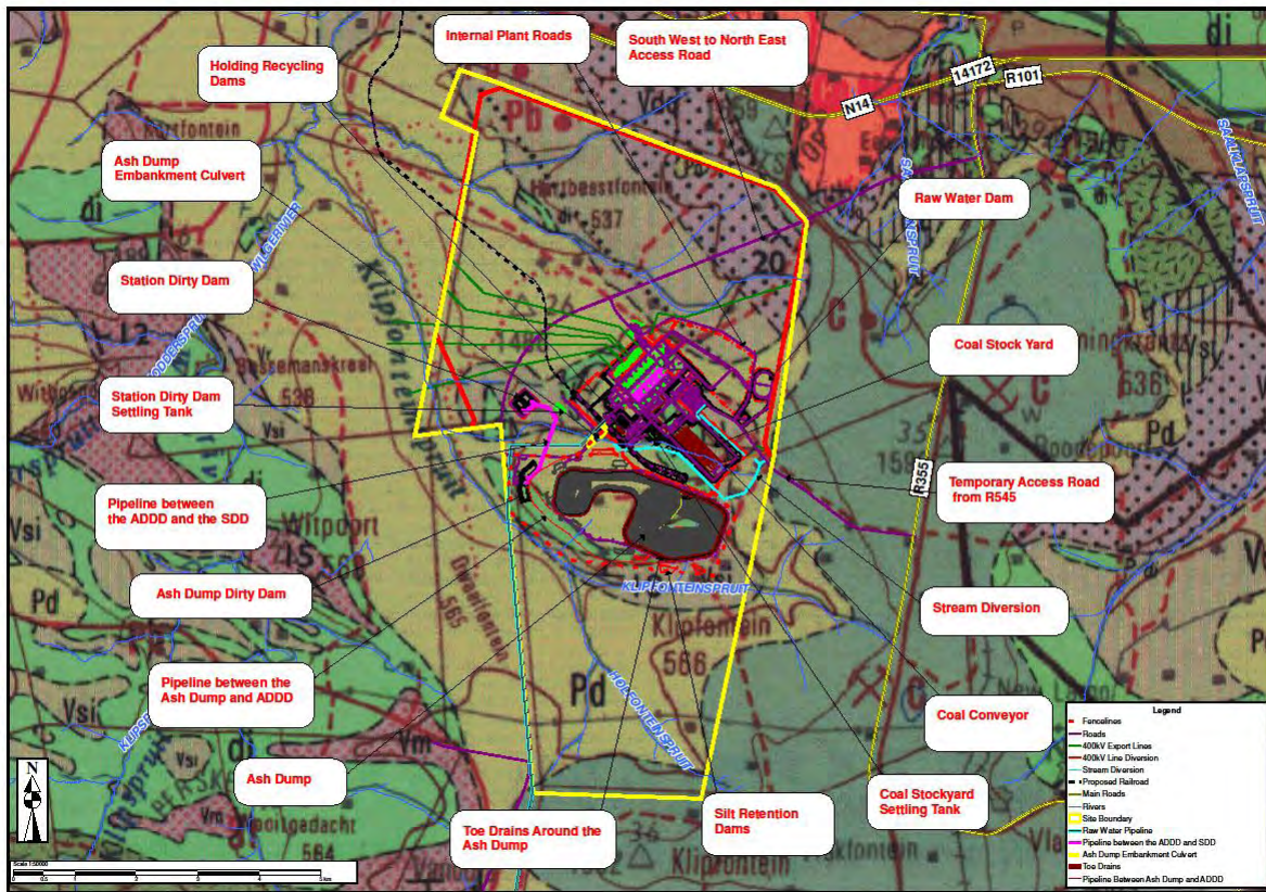
Figure 2: Geological map showing the position of the proposed ash dump of the Kusile Power Station in relation to the regional geology.
