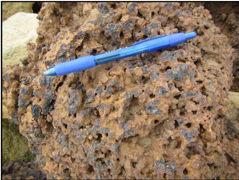
Figure 20: Clos-up view of the texture of the ferricrete present within the area (waypoint K002, see Figure 5).
