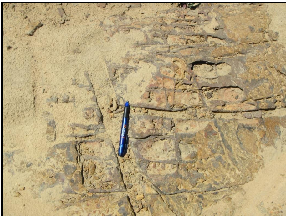
Figure 18: Fine- to medium-grained, maroon coloured sandstones lying stratigraphically higher in the sequence than the main, buff coloured sandstone that forms the prominent kran's in the region. The unit is extensively jointed and the margins of the joints are more heavily indurated than the remainder of the rock
