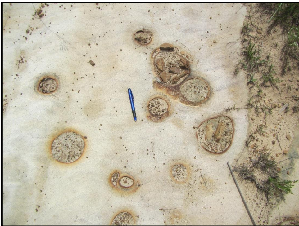
Figure 16: Hollow concretions with iron-enriched mantles within the Vryheid Formation sandstone (waypoint K010, see Figure 5).
