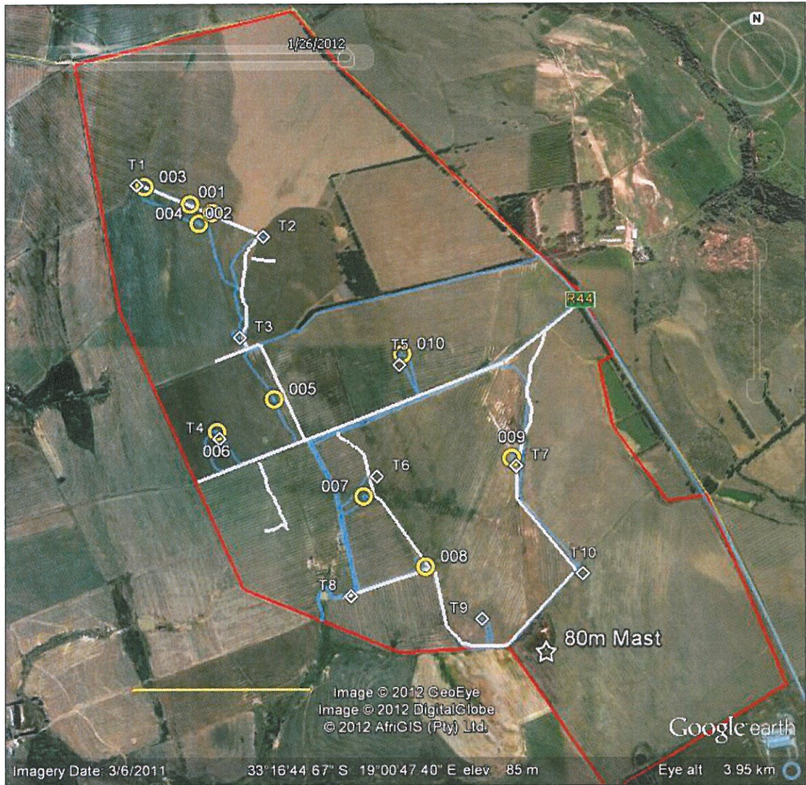
Figure 8: Aerial view of the study area showing the position of tracks paths (blue lines), proposed roads, (white lines), proposed turbines (white diamonds) and archaeological finds (yellow circles). Tree lines are obvious as dark lines and not labelled on the image.
