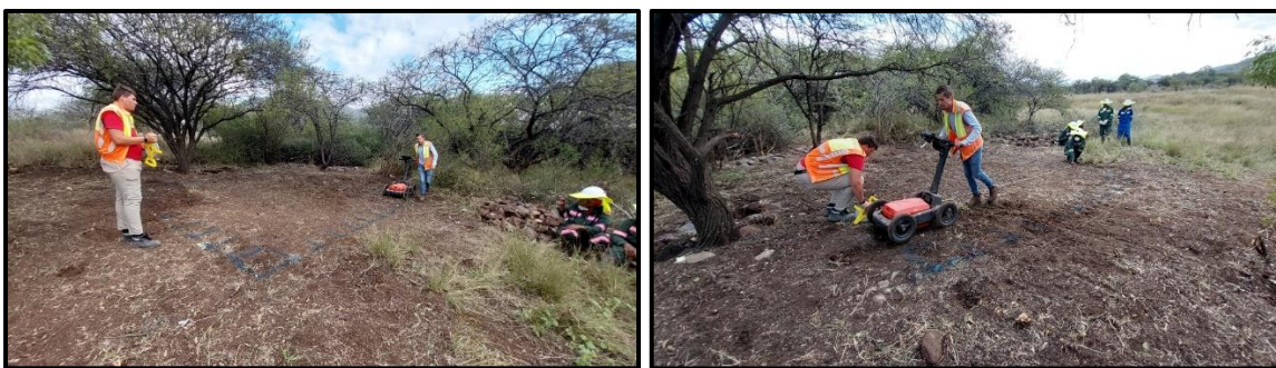
Figure 3.28. Image showing the GPR scanning process.
