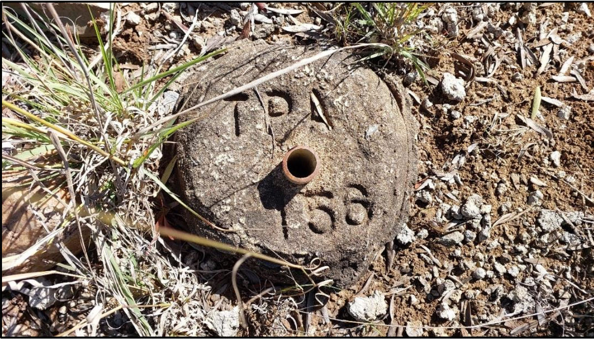
Figure 3.6. Image showing the cement marker.
