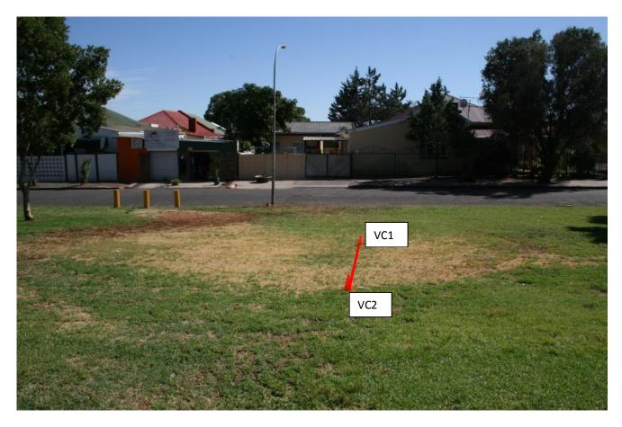
**Marked position VA1.** The GPR image suggests buried objects are present in this area; it can well be an old rubbish dump or building rubble.
