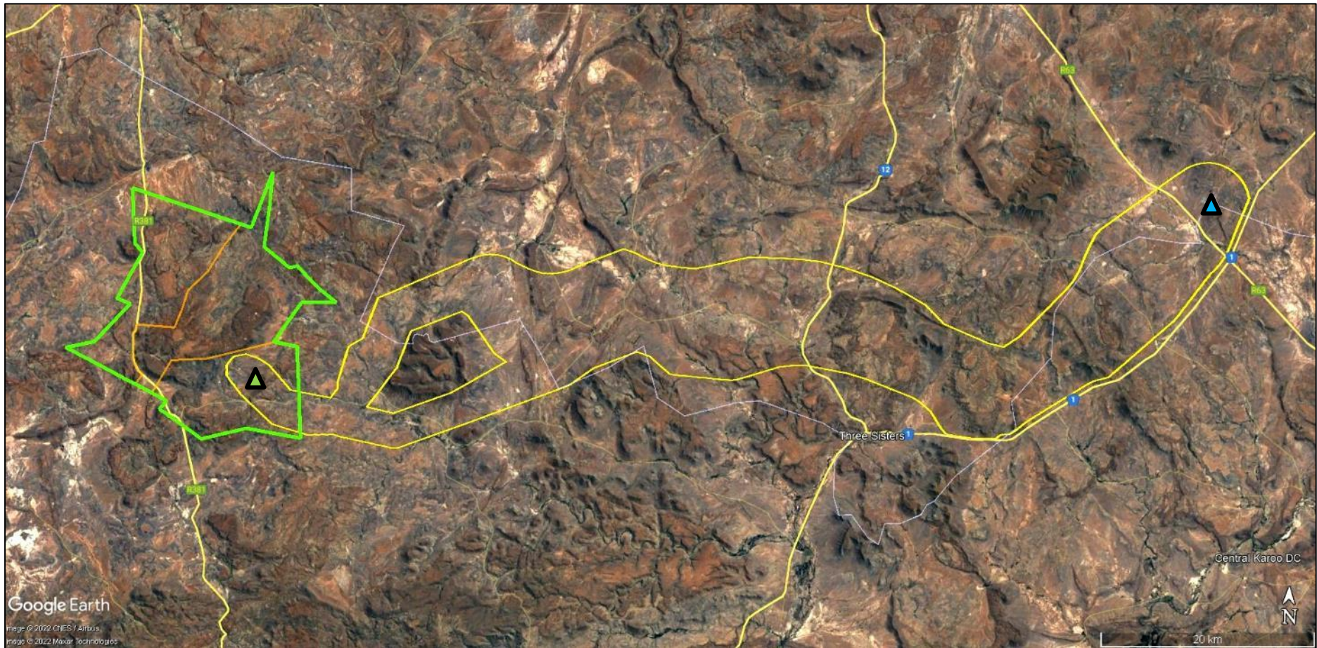
Figure 5-3: Google Earth© satellite map of the proposed Gamma Gridline Corridor (yellow polygon) between the Nuweveld Collector Substation (green triangle), located within the Nuweveld Wind Farm (green polygon) project area near Loxton, and the existing Eskom Gamma Substation near Hutchinson (blue triangle) some 90 km to the east. The corridor encompasses a range of semi-arid, hilly to mountainous terrain as well as low-lying alluvial vlaktes within the Upper Karoo region between Loxton and Beaufort West. Areas featuring major dolerite intrusions appear rusty-brown here.
