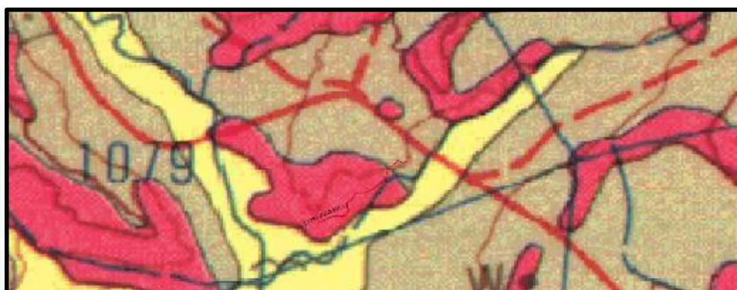
Figure 2 Geology underlying the proposed upgrade includes rocks of the Volksrust Formation (grey) and dolerite (pink). Site indicated as a thin red line on the map
