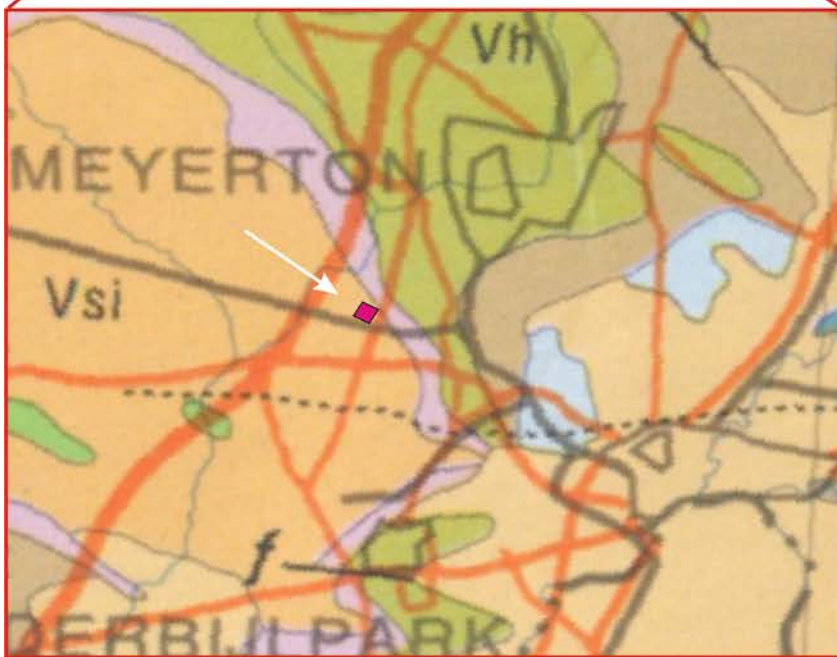
Figure 3. Portion of 1: 1 000 000 geological map of South Africa (Council for Geoscience, Pretoria) showing the geology of the proposed development footprint near Sebokeng. The study area is underlain by mudrocks of the Silverton Formation ( Vsi ). Volcanic rocks of the Machadodorp Member ( Vh , green) and sandstones of the overlying Magaliesberg Formation ( Vmg , purple) crop out to the north and east of the study area.
