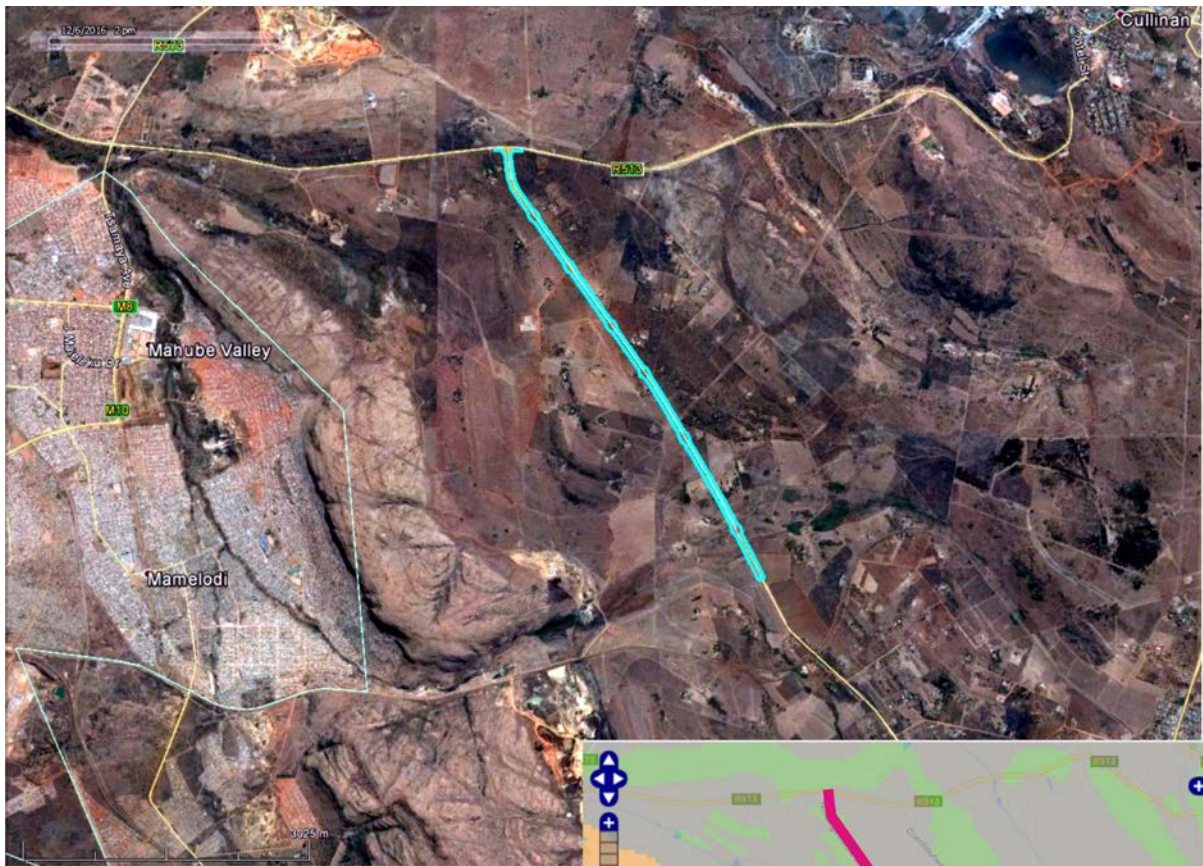
Figure 2. Aerial view of the road section (top). The is primarily underlain by diabase intrusions (SAHRIS Palaeo-sensitivity Map, grey areas, right insert) and to a very small degree by Transvaal Supergroup sandstone and shales (SAHRIS Palaeo-sensitivity Map, green areas, right insert).
