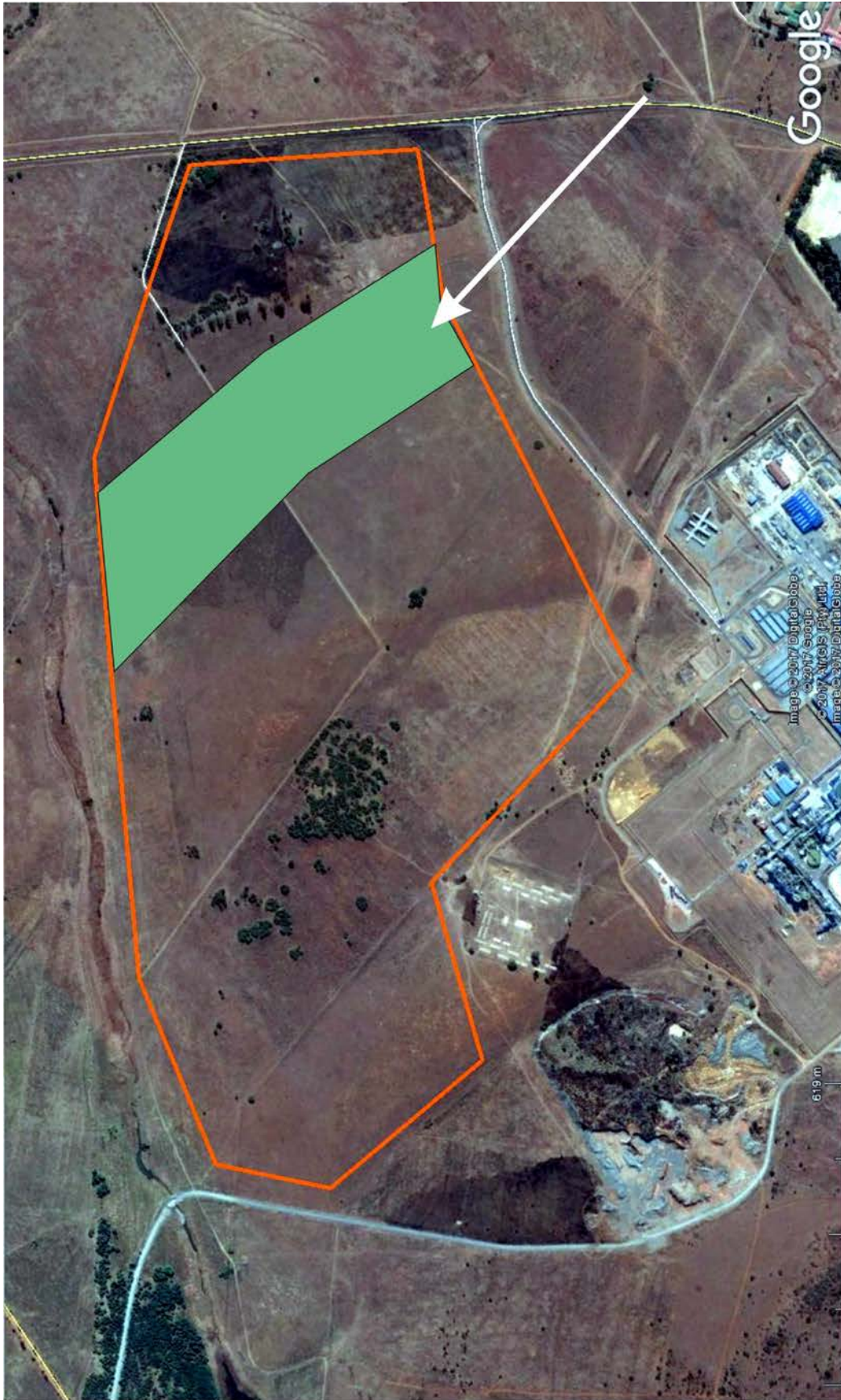
Figure 4. Estimated position of diabase intrusion contact zone according to the 1:250 000 scale geological map 2626 Wes Rand.
